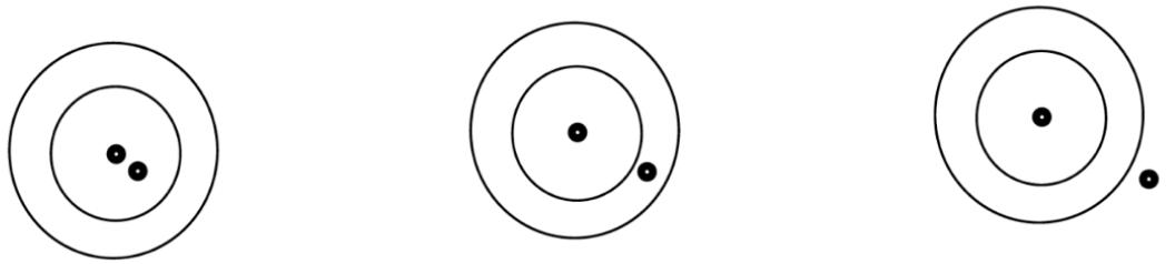
Beam Alignment $<1.5^0$     $1.5^0 <$  Beam Alignment $<3^0$    Beam Alignment $>3^0$
