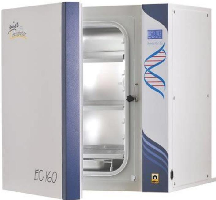
**Slika 4.** Prikaz CO<sub>2</sub> inkubatora Nuve EC 160
