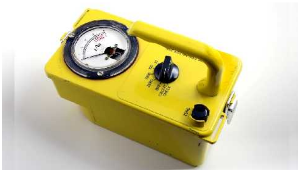
Slika 17. Geiger – Mullerov brojač (Izvor: https://www.livescience.com/how-a-geiger-counter-works.html )
