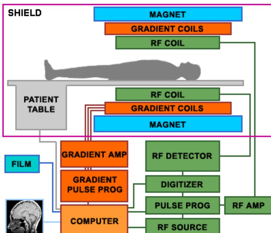
Slika 1: Građa MR uređaja (izvor: <https://eeoprojectz.blogspot.hr/2015/07/how-magnetic-resonance-imaging-mri-works.html>)
