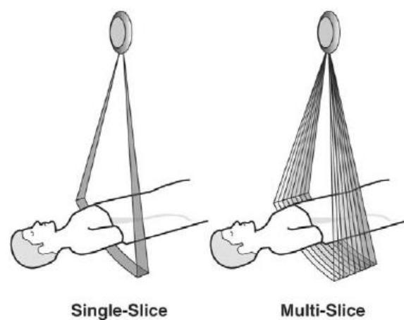
Slika 7. Shematski prikaz MSCT-a; izvor: [https://www.researchgate.net/figure/8333271\\_fig3\\_Fig-3-Comparison-of-single-slice-and-multislice-CT-scanner-A-single-slice-CT-scanner](https://www.researchgate.net/figure/8333271_fig3_Fig-3-Comparison-of-single-slice-and-multislice-CT-scanner-A-single-slice-CT-scanner)
